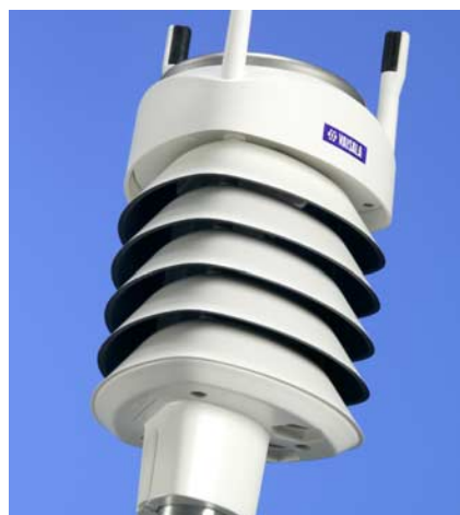
Barometric pressure, temperature and humidity sensors are combined in an advanced PTU module placed inside the specially designed radiation shield.
